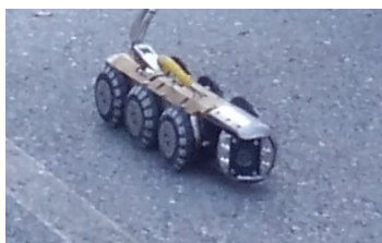
CCTV Sewer Camera, with rubber tire set-up for 8-inch diameter pipes
