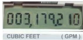
**Flow Rate**, in gallons per minute, becomes visible when the screen toggles. This screen displays for four seconds before toggling back to the "Read" screen.
